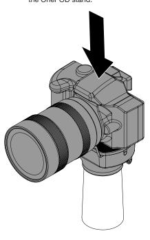
Place a charged and coded OneKEY against the lens on the side of the camera sensor. Press the button on the key to transfer the store's code to the sensor.
