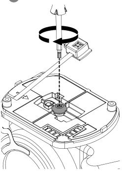
Attach the camera lens that is to be displayed.
