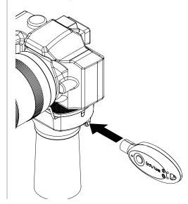
Remove the sensor and device from the stand. Place the magnet key (DBG400 or DBG406) into the depression on the sensor and push it inward to release the sensor cable. Pull the cable free.
