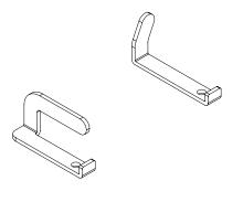
Insert the anti-rotation bracket, whichever best matches the shape of the camera, into the bottom of mounting plate.
