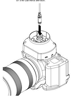
Place the camera and sensor onto the OnePOD stand.
