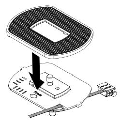
Place the mounting plate assembly onto the bottom of the camera. Align the screw on the plate with the hole in the bottom of the camera.
