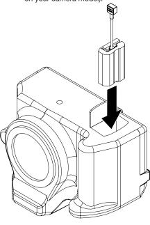
Route the cable out the side of the battery bay (some cameras may have a flange or trapdoor to aid this). Close the battery door.
