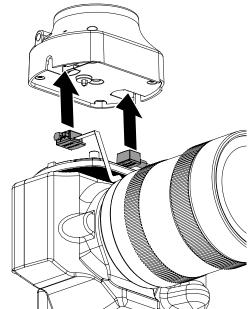
9 Insert the 2 screws into the bottom of the sensor housing.
