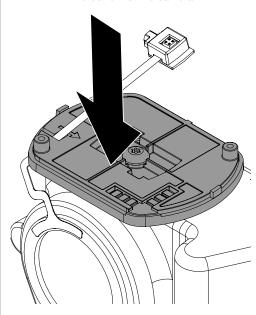
Tighten the screw using a TT20 bit.
