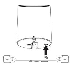
If routing power cable above fixture, route power cable out the back of the stand.
