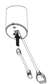
If routing power cable below fixture, route power cable through slot.
