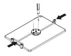
Use T20 bit to tighten the 3 screws on bracket hands. Do not overtighten or damage may occur to the device.
