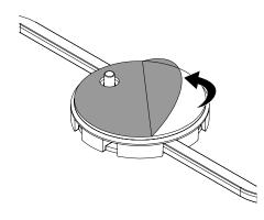
Position the mounting plate with the viper arm facing the power port on the device. Place mounting plate onto the center of the back of the device. Confirm bracket arms do not interfere with the power port. Press mounting plate firmly against the tablet for at least 10 seconds.
