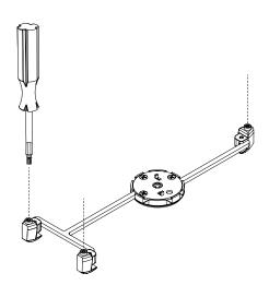
Remove clear film from the adhesive on the mounting plate.
