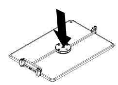
Slide bracket arms around the device. Use a Philips screwdriver to fully tighten the 3 screws on mounting plate.
