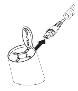
10 To remove sensor from device:
