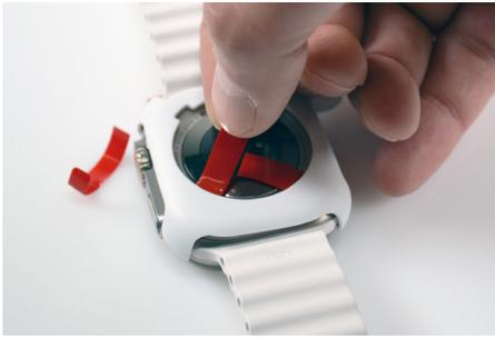
9 Flip the wearable over and pull the 3 red tabs out through the opening in the bottom of the tray sensor.
