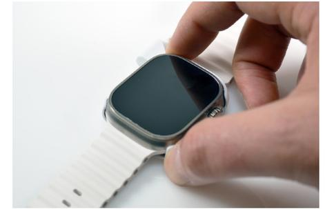
12 Press the adhesives on the tray sensor against the wearable for at least 10 seconds.
