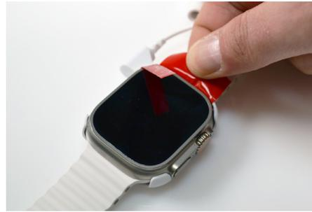
10 Pull the red tab for the adhesive along the bridge.
